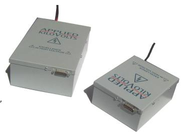
The LT Series builds on the new standard for high voltage precision and stability set by the LS 1 W family. By optimising the Low Stress™ technologies pioneered in the LS family, the LT Series provides 3W o/p capability, but still has less than 2ppm ripple, 10ppm/°C temperature coefficient, and 75ppm drift/hr throughout the range, while retaining the same LS case dimensions. Each of the units includes a differential control input.
